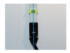
Should there be the need for further adjustment, simply turn the grub screw another 1/4 revolution clockwise, check alignment and so on, until the string is perfectly in the center of the bow.
