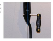
Tighten (clockwise) the opposite grub screw by approximately ½ revolution.
