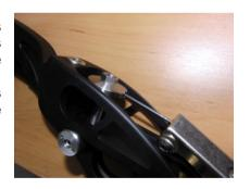
After having loosened the grub screw with a 2 mm Allen key, the limb screw can be adjusted by screwing outwards or inwards on the limb bolt. (14 mm key)
