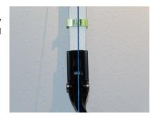
Loosen the grub screw (counterclockwise) in the center of the lateral adjustment at that side, the limb is pulling to by 2-3 revolutions. In this example it is the right side. Use a 3 mm Allen key.
